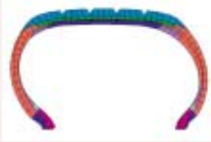
TIRE SECTION SHOWING DIFFERENT MATERIALS
