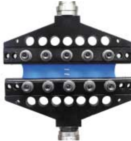
PLANAR SHEAR TEST WITH LASER REFLECTION TAGS
